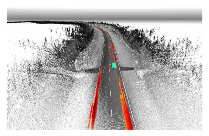
Figure 3. Example of a point cloud video of deformations in pavement surface (red) and locations with roughnes problems (blue). In the future this data could be viewed by a pavement engineer in a moving car but also truck drivers, for instance, could be warned about problem sections using this technique.
