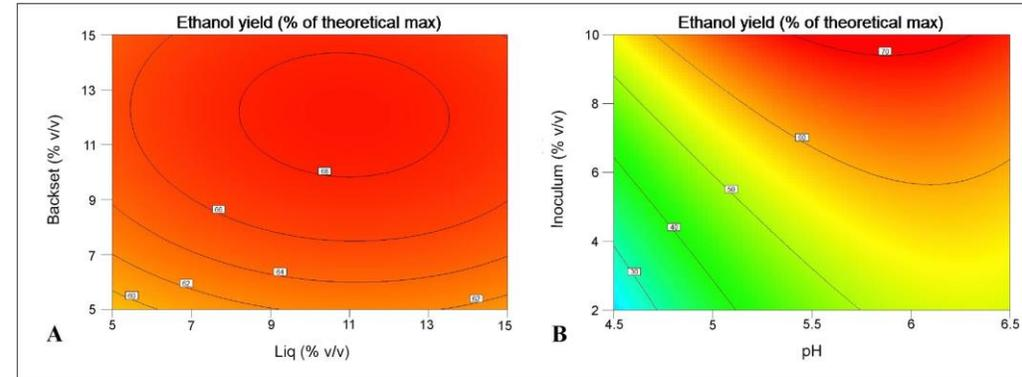
**Prediction of the optimum areas** for maximizing ethanol yield values as a function of backset and liq. addition (**A**) as well as the initial pH and inoculum volume (**B**). Maximizing the ethanol yields from hemicellulosic hydrolysate (**C**).
